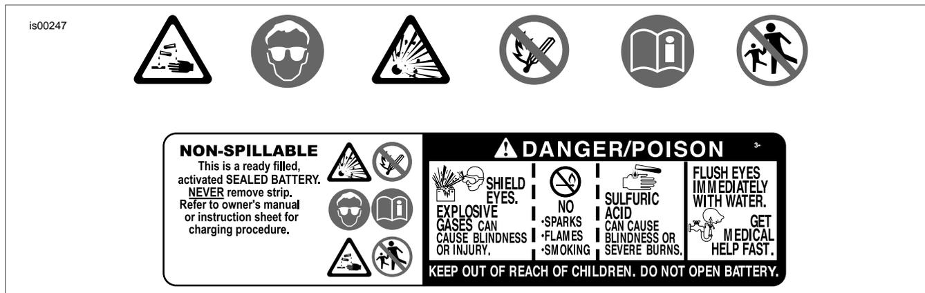
Figure 1. Battery Warning Label
